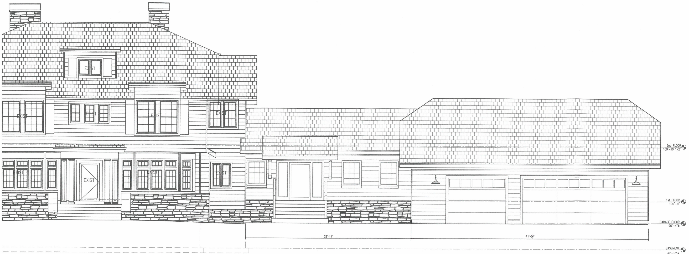
FRONT ELEVATION SCALE: 1/4"=1'-0"
